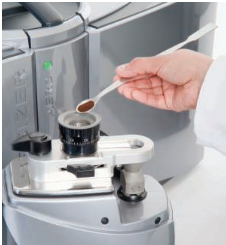
FIGURE 1. By enabling the close control of dispersion conditions during measurement, a laser diffraction system generates accurate particle-size data and also allows an assessment of the propensity of catalyst particles to undergo attrition
