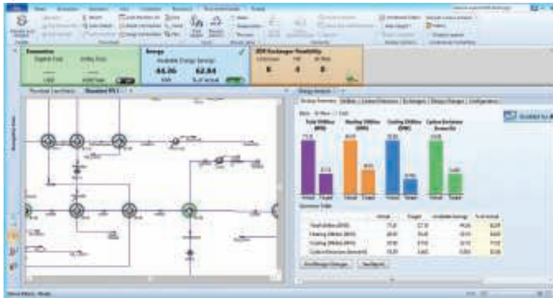
FIGURE 2. Among the tools offered for integration with aspenONE Engineering and Aspen Plus for modeling and simulation are Aspen Energy Analyzer (shown here), Aspen Economic Evaluation, Aspen Equipment Design and Rating and Aspen Basic Engineering
