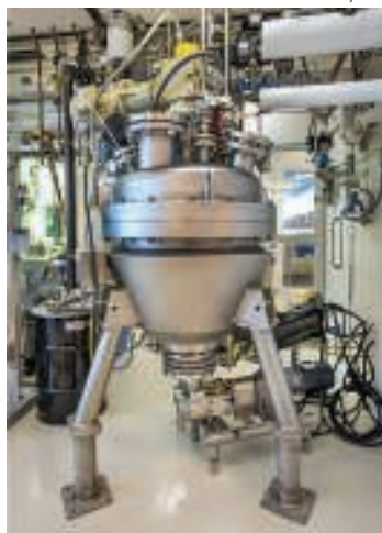
FIGURE 1. JBEI has scaled up biomass pretreatment technologies that utilize ionic liquids from the bench scale to the 100-L scale using a reactor located at the Advanced Biofuels Process Demonstration Unit (ABPDU)
